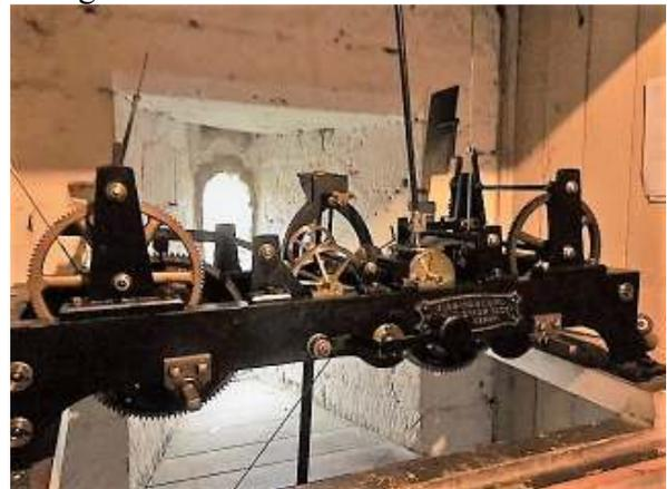
Winding the clock manually involved using a large handle to raise three weights at least once a week; the clock would run for up to seven days before it needed to be wound but it was easier to wind it twice a week as two of the weights (for the chime and for the strike) are in excess of 2½ hundredweight! It was a good workout!
